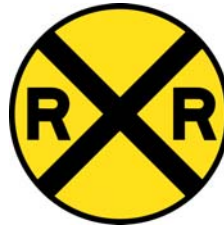
Figure 10-3. Railroad Crossing Advance Sign.
